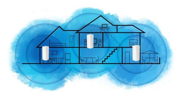
Another advantage of a mesh system would be that less Ethernet wires are required for each router, allowing the network to be truly "wireless". Furthermore, the additional child routers will be automatically configured once linked to the main node and will allow the user adaptability as more or less coverage is required in the property.
