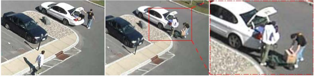
Figure 2.4: Representative frames of global and local activities recognized in this work. The first frame shows a person approaching a vehicle (global activity). Low resolution motion features are suitable for recognition of such actions. The second frame shows a person loading a trunk. This is a local activity which can be recognized by examining high resolution motion features in the region marked in red (showed in the third frame).
