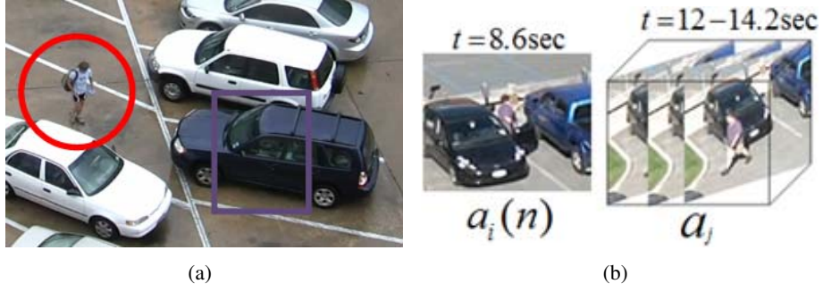
Figure 3.3: (a) The image shows an example of inter-activity spatial relationship. The red circle indicates the motion region of a_i at this frame while the purple rectangle indicates the activity region of a_j . Assume SC is defined by quantizing and grouping r_s(n) into three bins: r_s(n) \leq 0.5 ( a_i and a_j is at the same spatial position at the n^{\text{th}} frame of a_i ), 0.5 < r_s(n) < 1.5 ( a_i is near a_j at the n^{\text{th}} frame of a_i ), and r_s(n) \geq 1.5 ( a_i is far away from a_j at the n^{\text{th}} frame of a_i ). In the image, r_s(n) > 1.5 , so, sc_{ij}(n) = [0 \ 0 \ 1] . (b) The image shows one example of inter-activity temporal relationship. The n^{\text{th}} frame of a_i occurs before a_j . So, tc_{ij}(n) = [1 \ 0 \ 0] .
