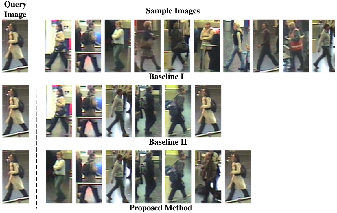
Figure 4.7: While Baseline I takes 148 (the first 10 are shown only) and Baseline II takes 6 sample images, the proposed method is close to Baseline II taking 7 sample images to label the query image. The attribute ‘hasbackpack’ helps to reduce the labeling effort here.
