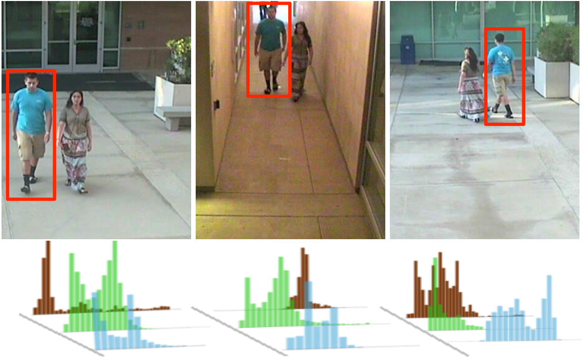
Figure 1.2: Three images of the same person in three non-overlapping cameras from the RAiD dataset [21]. Below each image, HSV features are shown as 3 different histograms. Brown denotes the hue, green denotes saturation and the sky-blue denotes the value histograms respectively. The inconsistency of the histogram shape does not allow them to be used as unique features for re-identification.
