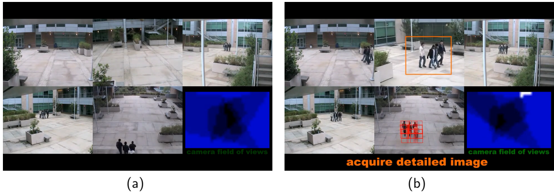
Figure 6.13: A group of people enter the area and a high resolution image of the entire group is taken. (a) Shows the initial coverage of the camera network. The blue shaded region shows the area coverage of the current camera settings. Lighter regions indicate less overlap in FOV. (b) Shows the resulting views and area coverage after one camera in the network self selects to acquire a high resolution image of the targets being tracked. Detections are shown as red boxes in the bottom middle camera.
