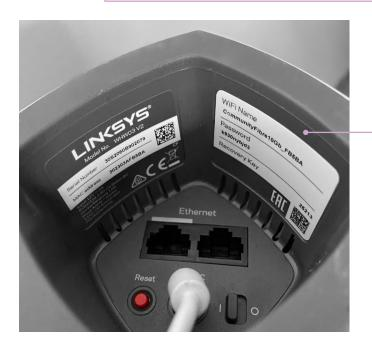
**Note:** Your Router Password will be located on the sticker in the underside of your main router.
