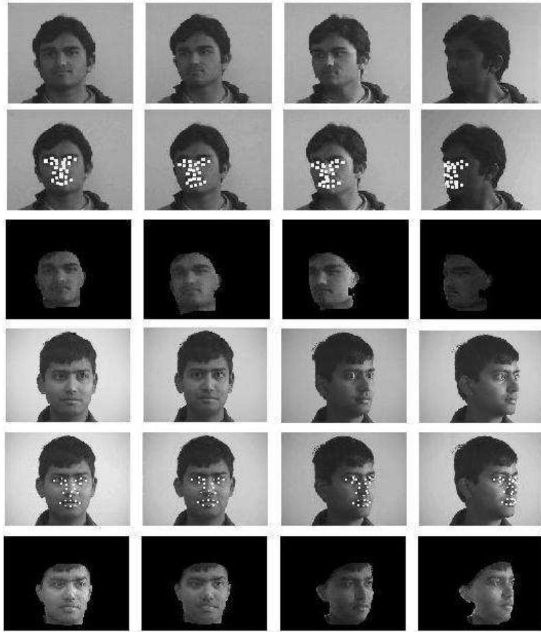
Figure 5.2: Original images, tracking and synthesis results are shown in three successive rows for two of the probe sequences.
