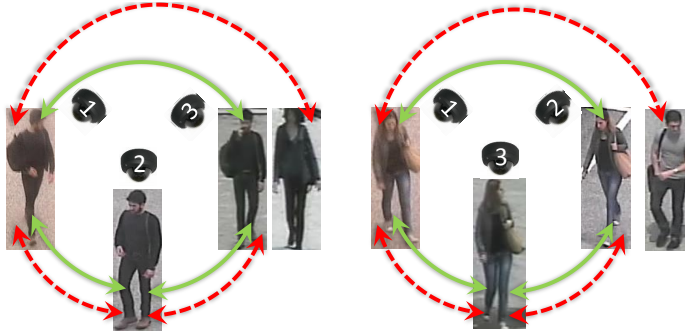
Figure 2.4: Two examples of correction of inconsistent re-identification from WARD dataset. The red dashed lines denote re-identifications performed on 3 camera pairs independently by FT method. The green solid lines show the re-identification results on application of NCDA on FT. The NCDA algorithm exploits the consistency requirement and makes the resultant re-identification across 3 cameras correct.
