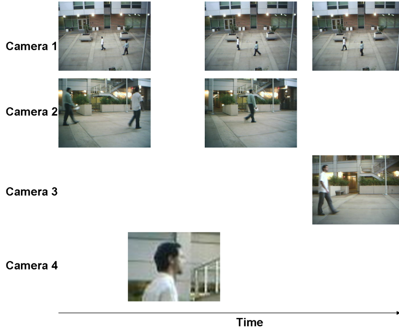
Figure 4.1: An example of a camera network where different cameras work collaboratively to fulfill different tasks. While Camera 1 keeps the entire scene in focus, it cannot get high resolution features on any of the people. This is done by Cameras 2, 3 and 4, but they have narrow FOVs. In fact, we can see that Camera 2 can no longer keep track of the person in the white shirt with its current settings, but can keep track of the other person. Camera 3, therefore, takes responsibility for tracking the person in the white shirt. With the information already available, Camera 4 is able to obtain a high resolution facial image.
